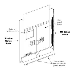
Dynaco Saf-T Egress Option: A T-shaped cut divides the door panel into 3 sections. The sections are held together by zippers. This allows the sections to release creating an emergency exit, simply by pushing at the indicated spot. The zipper is designed to break-away so it can immediately be released with minimal force. The dimensions of the egress passage are always 6.7ft high, with a standard width of door width minus 1.3ft. The passage width will vary with door installation.
