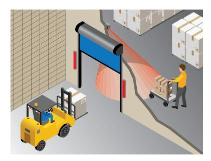
The Safe Pass can be programmed to operate via a variety of activation devices to give a red light signal even when the door is open if there is a person or object on the other side.
