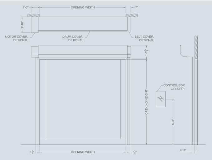
All indicated dimensions are minimum space requirements for installed door. Note: Based upon individual environmental safety considerations, extra safety components such as push buttons, detectors and covers may be required.
